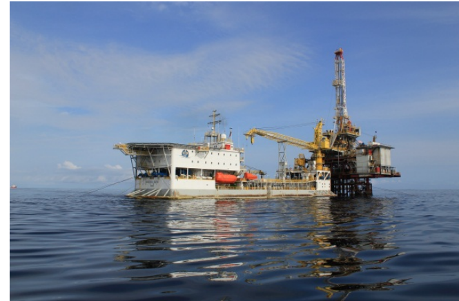
Flat bottom tender barges used on regions with relatively calm weather conditions, e.g. West Africa and SEA
