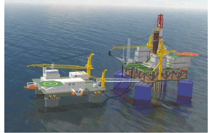
Tender semi required in regions with deeper water and more challenging sea conditions
