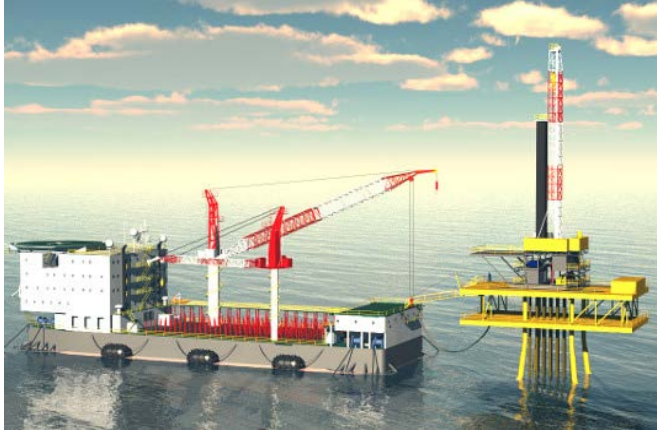
Tender barge used on fixed platforms
